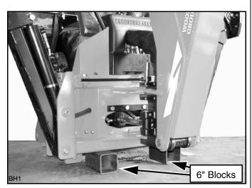
Figure 7. Backhoe Storage Position (Typical)
